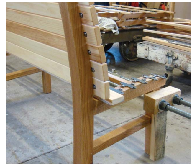
Pine being used for the slats and oak being used for the frame
